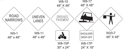
SIGNS SHOWN ABOVE ARE TO BE USED WHEN CONSTRUCTION OPERATIONS WARRANT. TO BE USED AS DIRECTED BY THE TDOT MANAGER.
